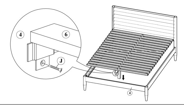
STEP 6 : Attach Assembled Bed Slats to Assembled Bed Frame with (F) Using a Allen Key M4 (A) as shown.
